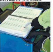
Everyday operations are streamlined using the barcode scanner. A barcode scanner allows operators to appropriate welding conditions and maintain the highest quality with just a simple scan.
